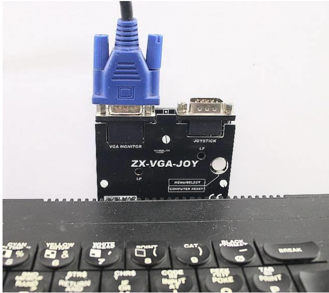
ZX-VGA-Joy, connected via a bus splitter.
